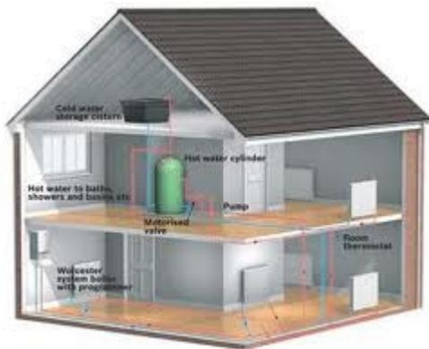
Your heating system basically consists of a heat source which can be in the form of an oil, gas or solid fuel boiler which is connected to a circulation pump. This circulates hot water which has been heating in the boiler around your house through the radiators and the coil of the hot water cylinder in the process before returning to the boiler to be re-heated again. The radiators heat your rooms while the coil in the hot water cylinder
